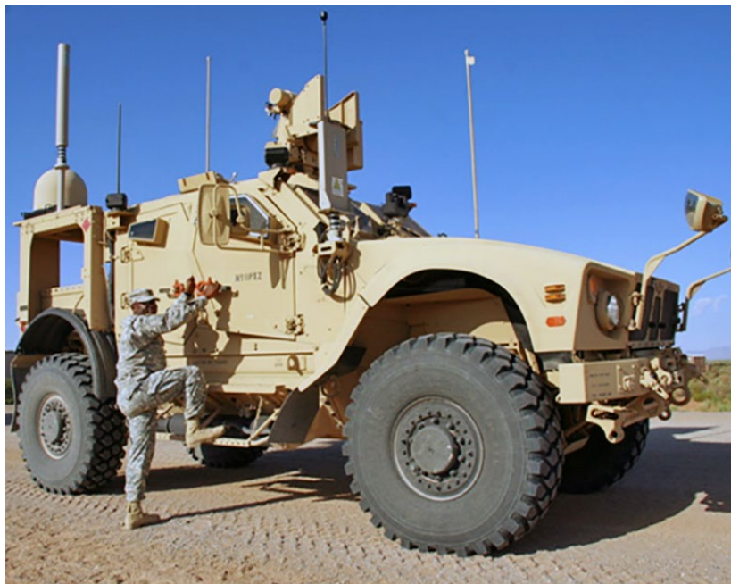
An NCO from 2nd Brigade Combat Team, 82nd Airborne Division, boards a Soldier Network Extension vehicle during the WIN-T Increment 2 developmental test in June. The vehicle provides network communication and extension capabilities at the company level. (Photo by Amy Walker)
