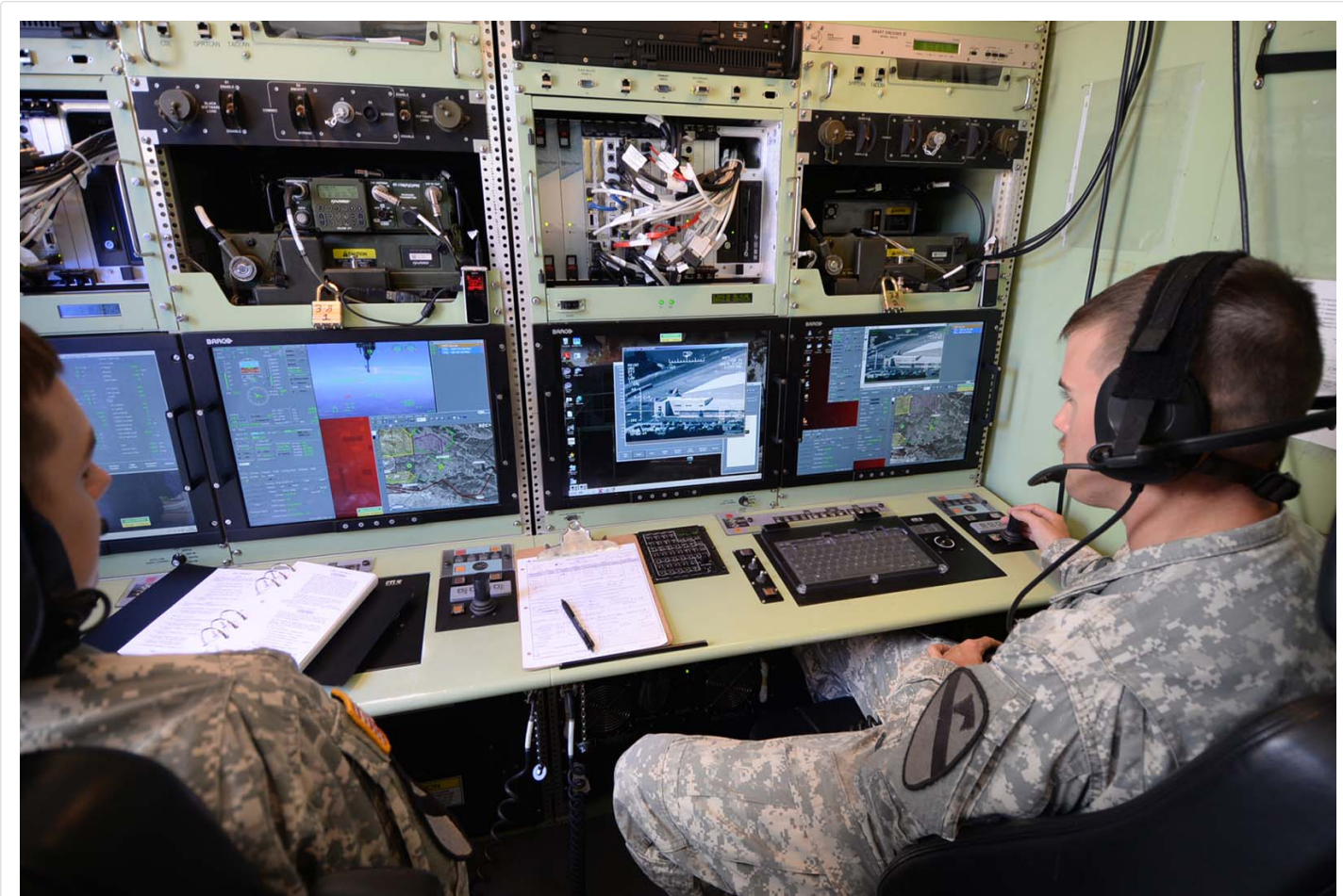
Gray Eagle UAVs are operated from within a ground control station. Spc. Zachary Zimmerman, left, works as the aircraft operator, while Staff Sgt. Mark Mushen controls the cameras and sensors as the payload operator. (Photo by Meghan Portillo/NCO Journal)
