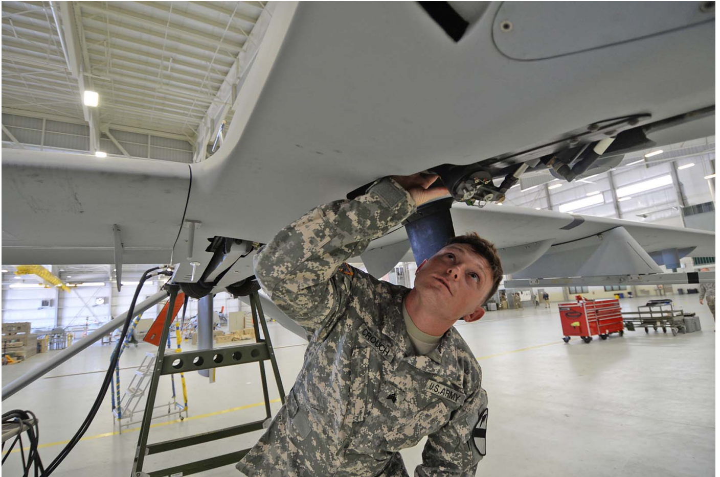
Sgt. Joseph Crouch, an unmanned aircraft systems repairer, performs preflight operational checks on a Gray Eagle UAV's landing gear. (Photo by Meghan Portillo/NCO Journal)
