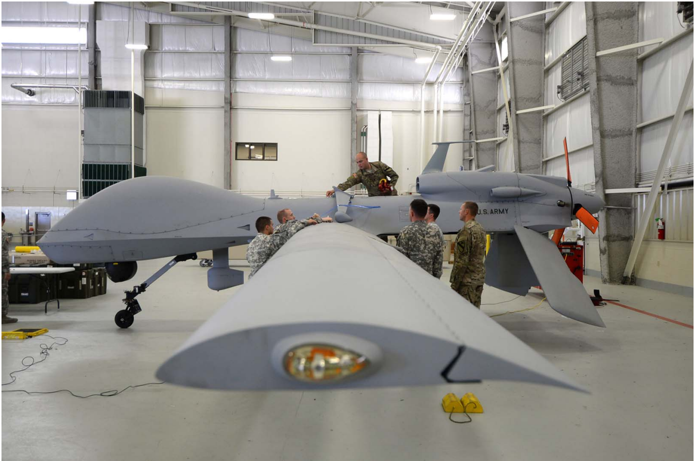
Sgt. Will Scott (top) and other unmanned aircraft systems repairers perform a preflight weight and balance check on a Gray Eagle UAV. (Photo by Meghan Portillo/NCO Journal)
