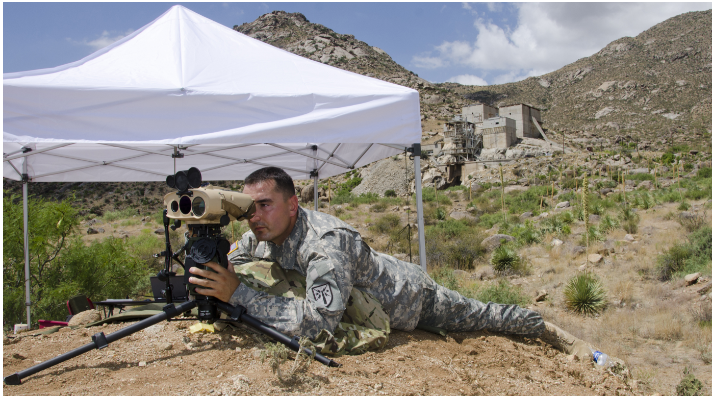
Sgt. 1st Class Justin Rotti, a combat developer for the U.S. Army Training and Doctrine Command Fire Cell, tests a developmental handheld precision targeting device for the Rapid Equipping Force in July 2014 at White Sands Missile Range, New Mexico. The device allows Soldiers to engage targets with precision munitions and provide digital connectivity to related units. (Photo by John Hamilton / White Sands Missile Range Public Affairs)
