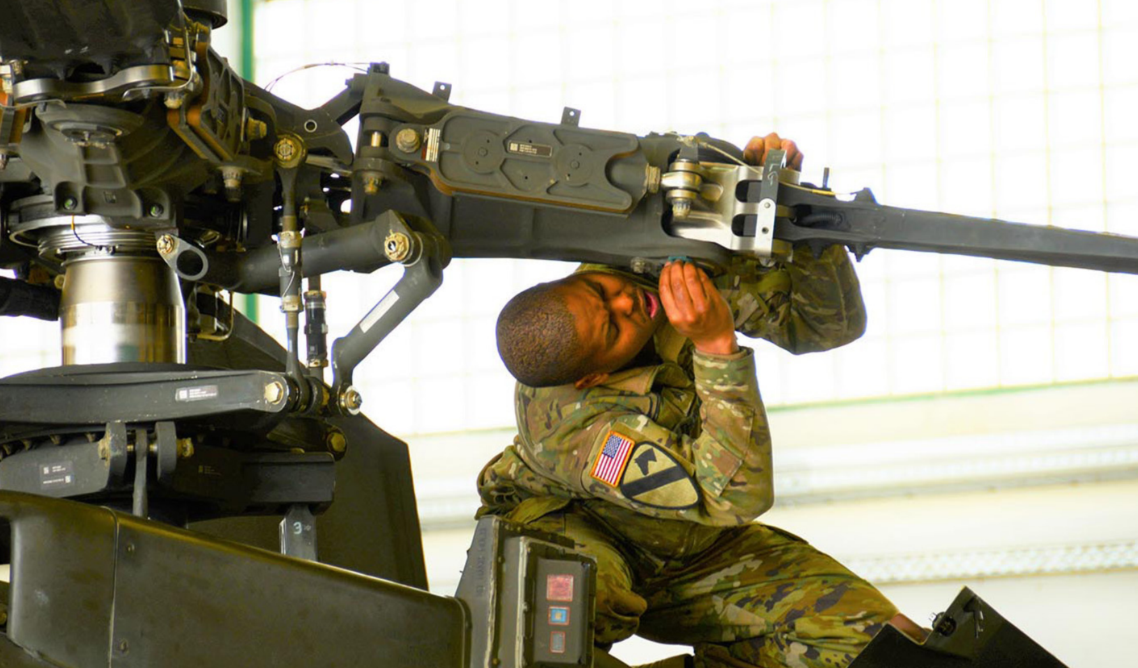
Sgt. Stefan Thorne, an Apache helicopter crew member from the 1st Battalion, 3rd Aviation Regiment (Attack Reconnaissance), 12th Combat Aviation Brigade, conducts phase maintenance on an AH-64 Apache helicopter on Oct. 3, 2017, at Katterbach Army Airfield in Ansbach, Bavaria, Germany. (U.S. Army photo by Charles Rosemond, Training Support Activity Europe)
