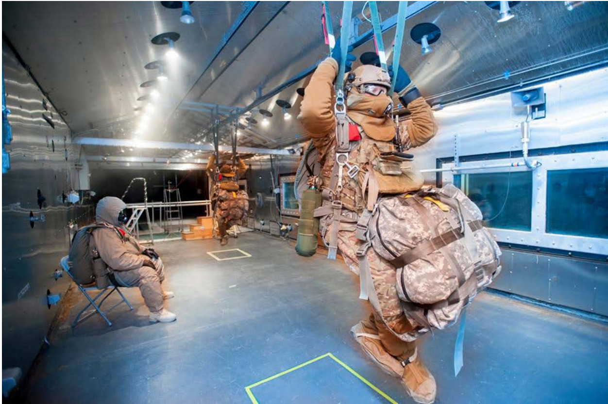
Noncommissioned officers help Aerial Delivery Directorate researchers test the RA-1 parachute's harness for comfort and fit in the Doriot Climactic Chamber's Arctic unit. (Photo courtesy of U.S. Army Natick Soldier Research, Development and Engineering Center)
