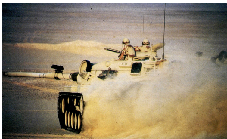
An M60/A1 kicks up a swirl of sand as it closes on its target. Dust clouds can obliterate a target or reveal its location. The sand is also an enemy to movement – clogging filters and stopping engines. (U.S. Army photo)
