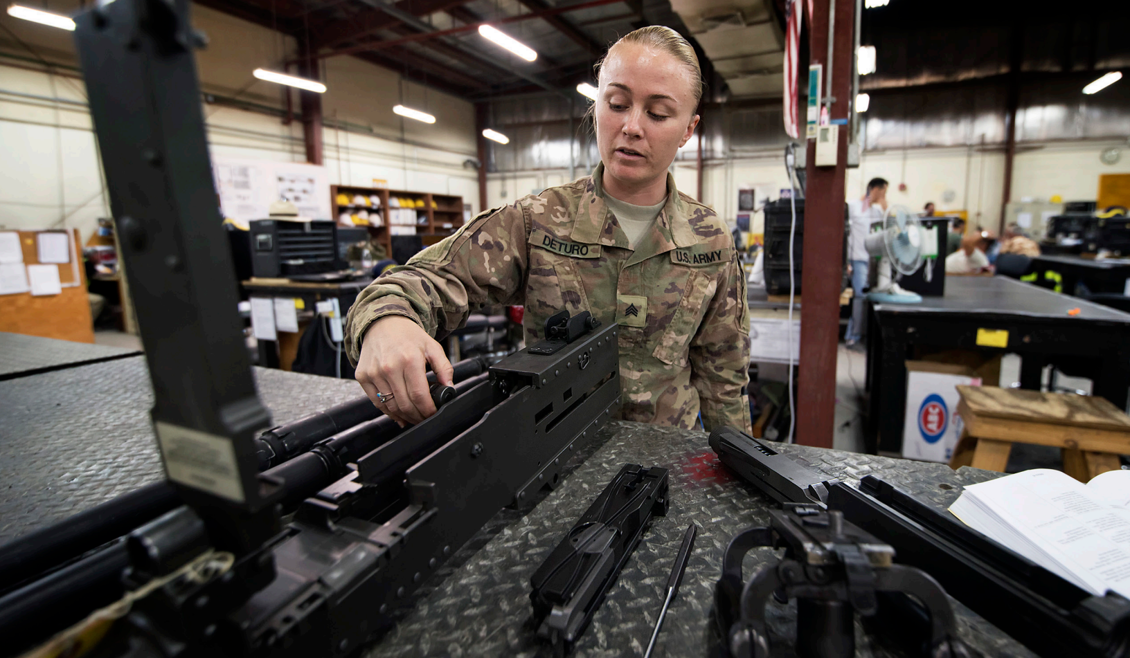
U.S. Army Sgt. Brittany Deturo, weapons quality assurance specialist with the 401st Army Field Support Battalion-Kuwait, checks the gap between the charging handle and the body of a M2 .50-caliber machine gun in the weapons maintenance facility of Army Prepositioned Stocks-5 at Camp Arifjan, Kuwait, Aug. 17, 2019. (U.S. Army photo by Kevin Fleming)
