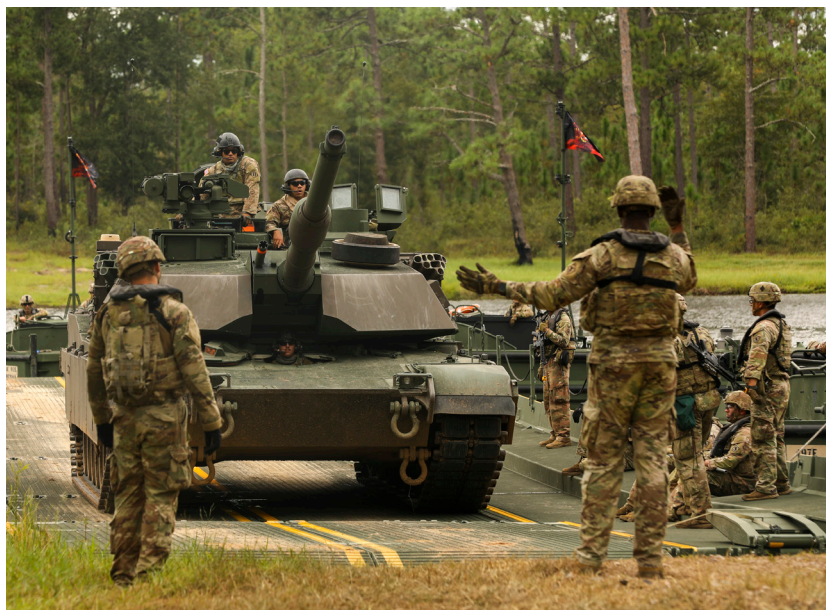
Soldiers assigned to the 497th Multi-Role Bridge Company (MRBC), 92nd Engineer Battalion, and 3rd Battalion, 69th Armor Regiment, 1st Armored Brigade Combat Team, 3rd Infantry Division, maneuver an M1A2 SEPv3 Abrams tank across an Improved Ribbon Bridge (IRB) during a wet gap crossing exercise at Fort Stewart, Georgia, Sept. 20, 2023. (U.S. Army Photo by Spc. Duke Edwards)
